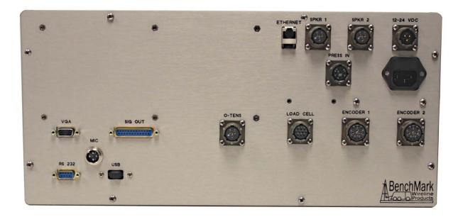
The system consists of two main components, the real time acquisition board and the PC. The acquisition board provides power to and processes the signals from the encoders, load pin, and magnetic mark detector. This board operates independent from the PC and is instantly on when power is applied. It also is connected to displays for depth and tension. This allows depth and tension to be displayed immediately on power up and always be displayed regardless of the PC status
